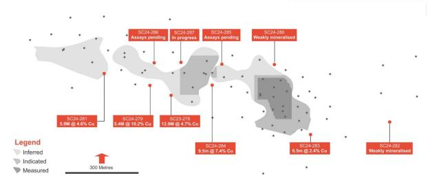
Figure 2: Plan of the Johnny Lee Lower Copper Zone at the Black Butte Project as of March 2024, showing current and past drill pierce points (red and black dots respectively) and resource domains (shades of grey)
