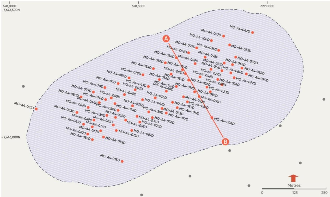
Figure 3: A4 Plan view – Collar location of drill holes used to inform the Mineral Resource. US\$4.50/lb Cu price optimised pit shell shown in dashed black outline. The position of cross-section A-B (Figure 2) is indicated.
