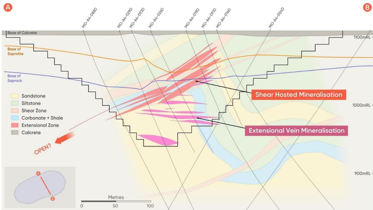
Figure 2: Schematic Cross-Section – showing interpreted geology and mineralisation styles across the A4 Deposit. US\$4.50/lb Cu price optimised pit shell used to constrain the Mineral Resource shown in black outline.
