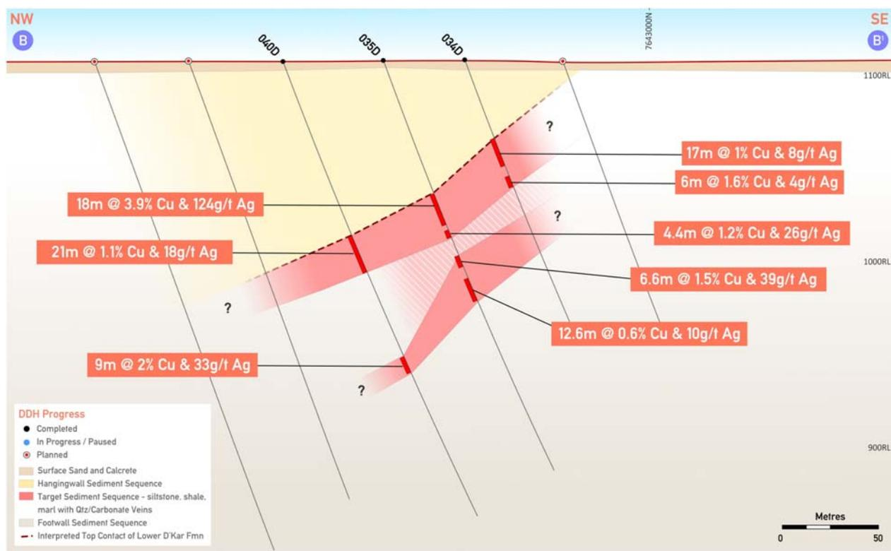
**Figure 4: Preliminary interpreted cross-section through MO-A4-034D, MO-A4-035D and MO-A4-040D located approximately 150m east from the section in Figure 3. (Note: this cross-section was included in the 17 April 2020 release).**
