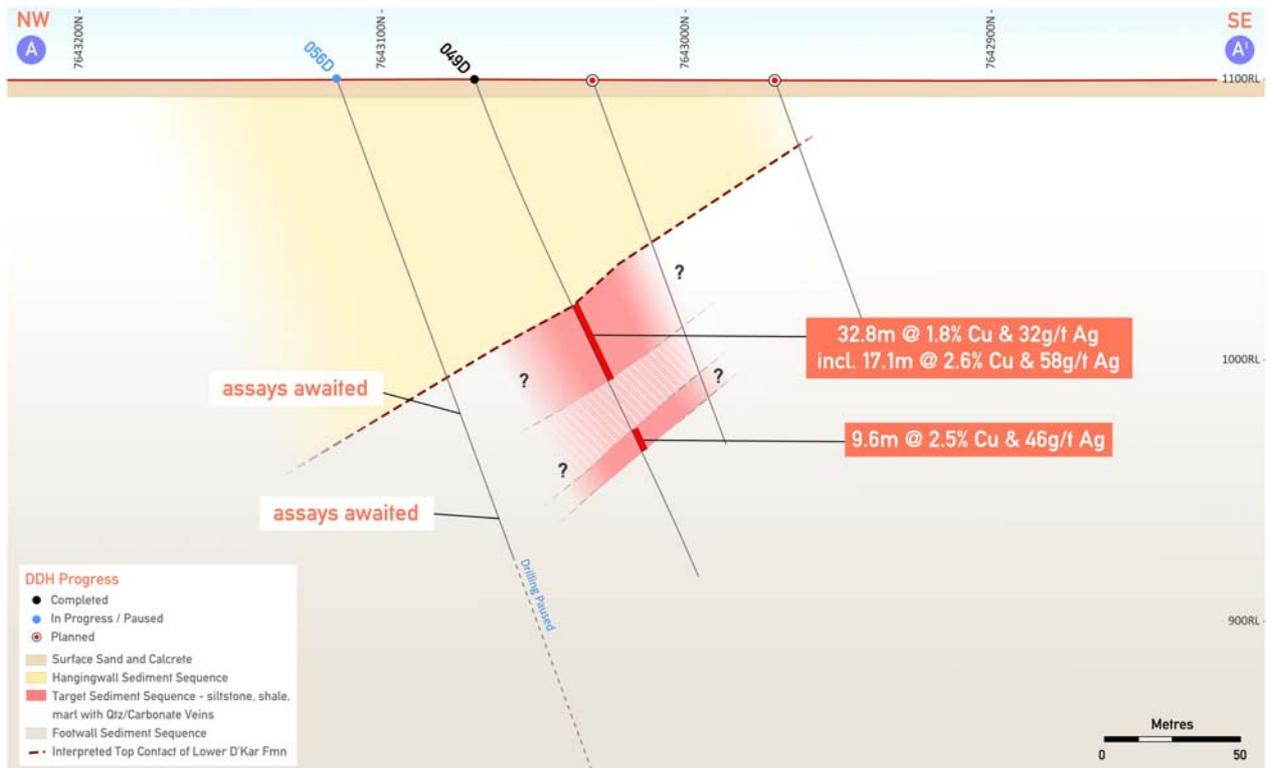
Figure 3: Preliminary interpreted cross-section through MO-A4-049D near the western limit of current drilling, showing completed and planned drill holes.
