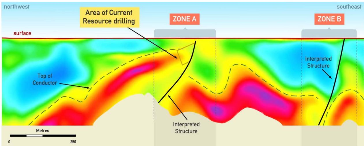
Figure 5: A4 CDI section – AEM data showing two zones of interpreted structural disruption (Zones A and B).
