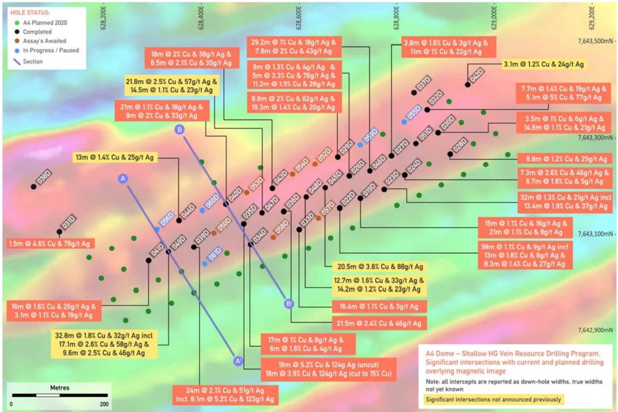
Figure 2: A4 resource drilling plan showing significant intersections from results reported in this release (yellow) and reported previously. Drill-hole collars plotted over magnetic image and locations of the two cross-sections (Figures 3 and 4) highlighted in blue.
