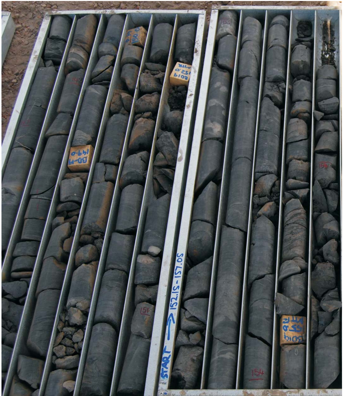
Very fine grained carbonaceous shale with fine pyritic sulphide bands
